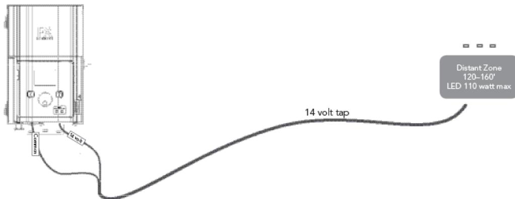
Watts shown are per 12 gauge cable. Install additional cable runs as needed to complete project. To increase wattage maximum, run 8 gauge or double 12 gauge to the first fixture in the zone. Use a digital voltmeter to fine tune circuits.
