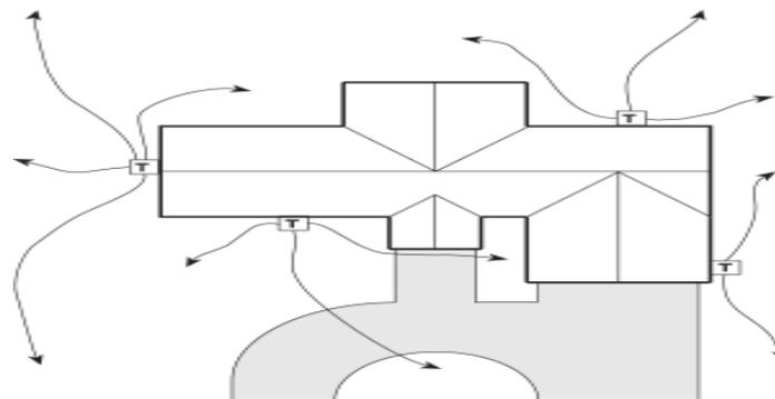
Sample diagram of home with transformer and lamp placement
